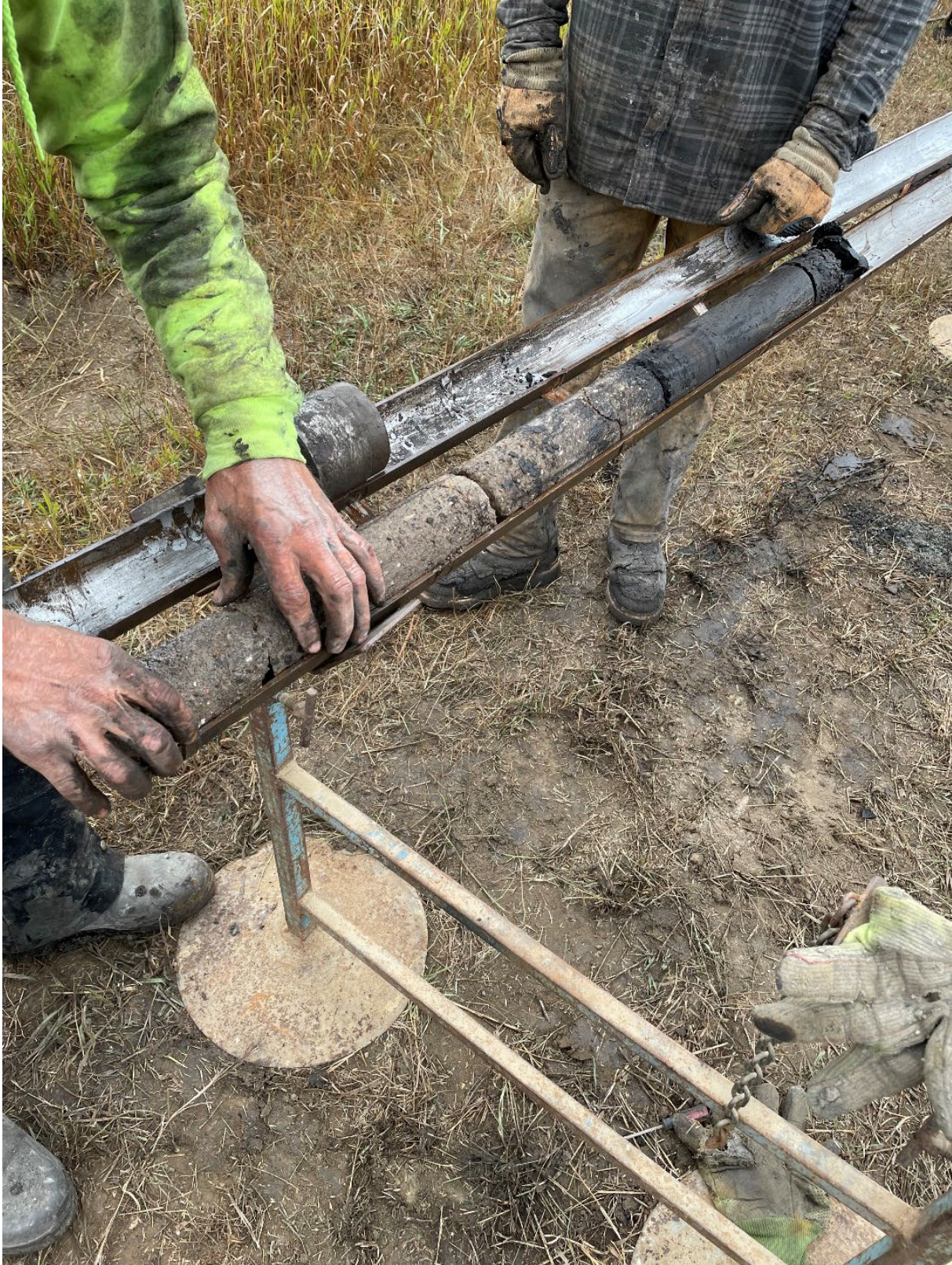
Figure 6: The drillers are opening the core barrel revealing solid grout and coal.
